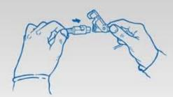
To prevent accidental or unauthorised use, each electrically powered, handset operated, chair incorporates a quick release feature. This is usually found on the lead inside the pocket at the side of the chair. Always detach the handset and store in a safe position out of the reach of children to prevent unauthorised or unsupervised use of the chair.
