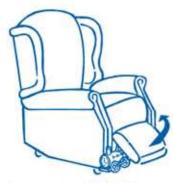
To prevent accidental damage or trapping when the footrest closes, each electrically powered chair incorporates a sprung-loaded footrest. Should the footrest hit an obstruction on closing, it will pivot as shown to reduce pressure.
